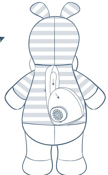
(EN): Remove sound unit from BACK opening to replace batteries.
