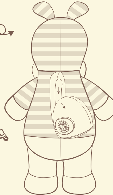
Remove sound unit from BACK opening to replace batteries.
